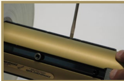
Each contact element moves up and down freely.
